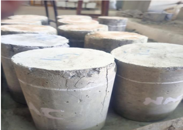
Fig. 4. Failure mode of unconfined RAC control specimen under axial compression (brittle splitting)
