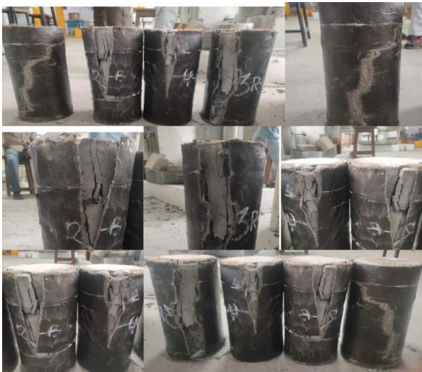
Fig. 6. Failure mode of BFRP-confined RAC specimen (uniform hoop cracking, fibre splitting)
