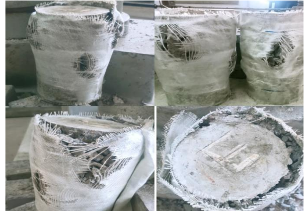
Fig. 5. Failure mode of GFRP-confined RAC specimen (longitudinal tearing, partial delamination)
