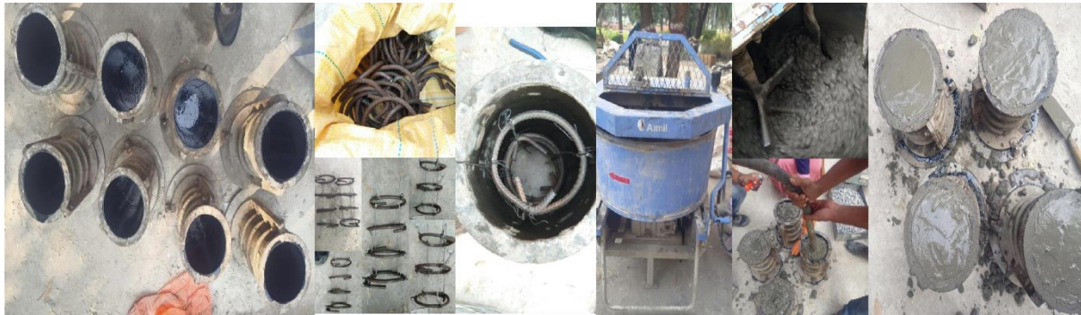
Fig. 2. Preparations of test specimens FRP sheets GFRP, BFRP, CFRP and confinement done
