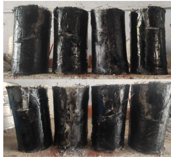
Fig. 7. Failure mode of CFRP-confined RAC specimen (mid-height rupture band, ductile behaviour)
