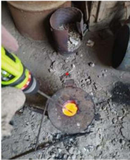
Fig. 2. The stir-casting technique
