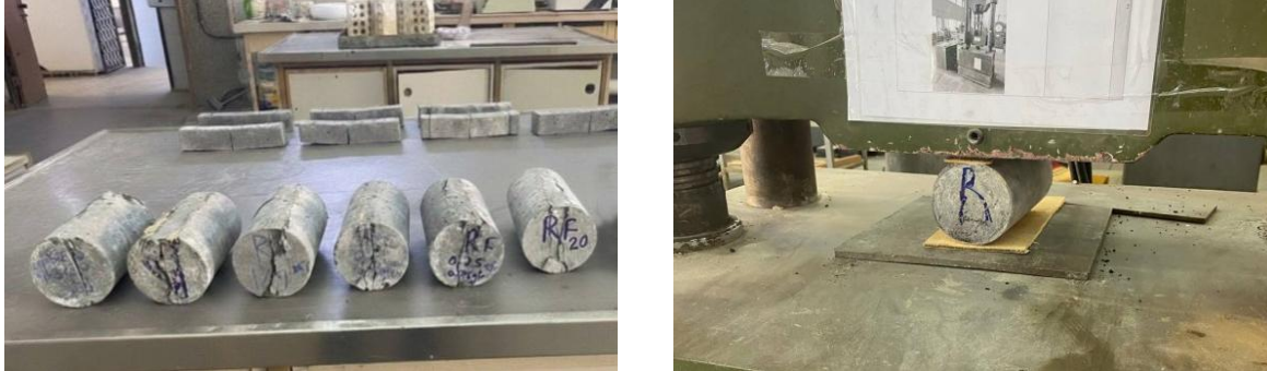
Fig. 6. Testing and failure of the specimens
