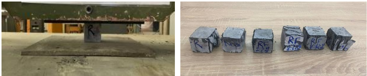
Fig. 4. Testing and failure of the specimens
