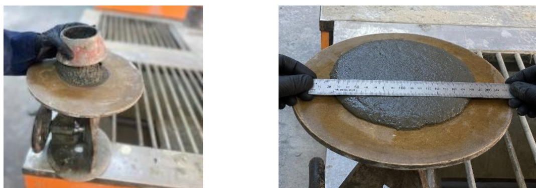
Fig. 2. Flow table test procedure
