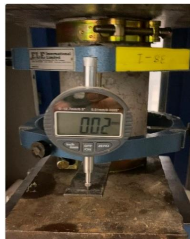
Fig. 3. Testing setup for the uniaxial compressive strength test
