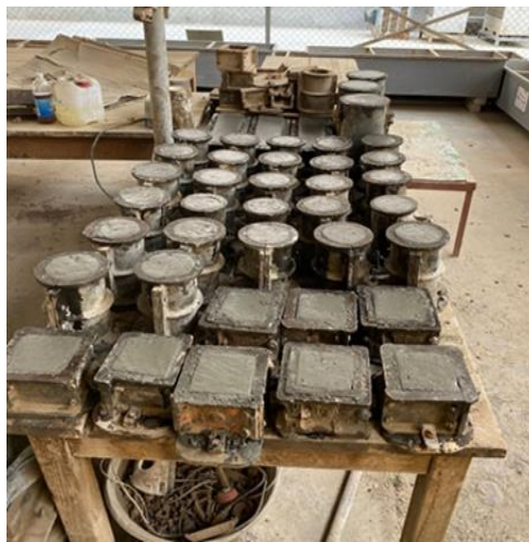
Fig. 1. Concrete specimens' preparation
