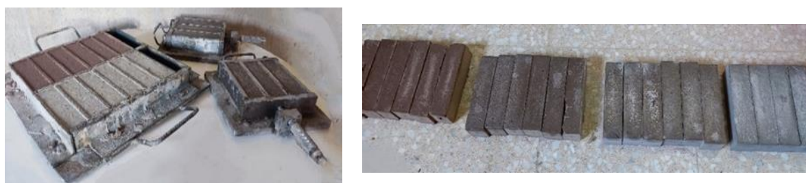
Fig. 5. Prepared mortar samples with different SSA substitution ratios
