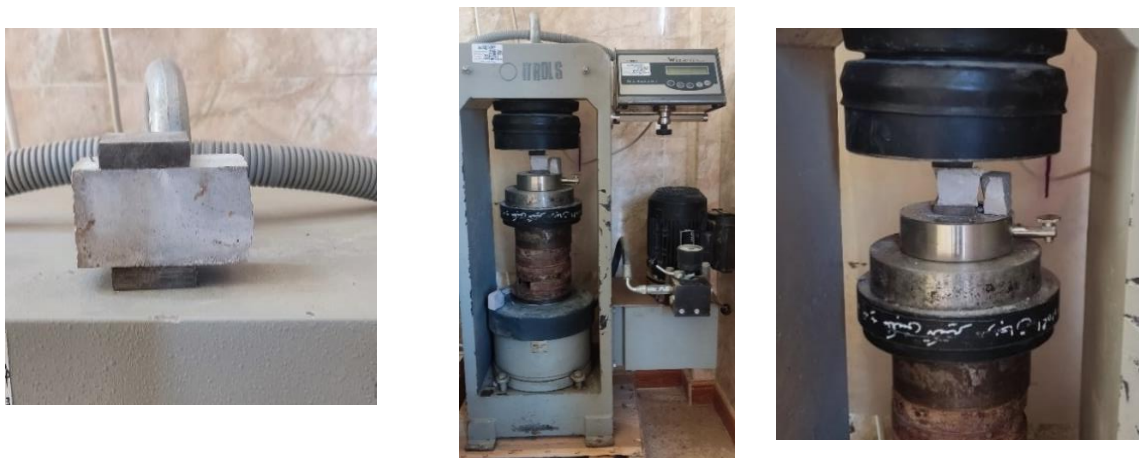
Fig. 7. Evaluating mechanical properties: focus on compressive strength testing
