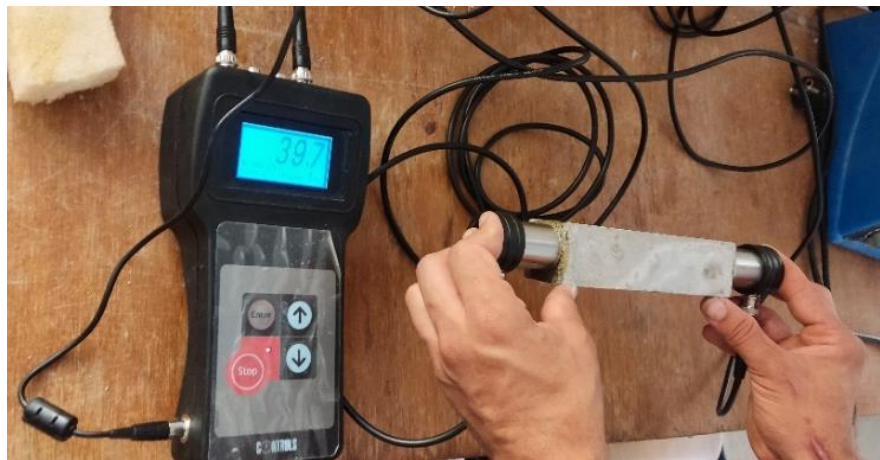
Fig. 16. Ultrasonic pulse velocity measurement in mortar specime
