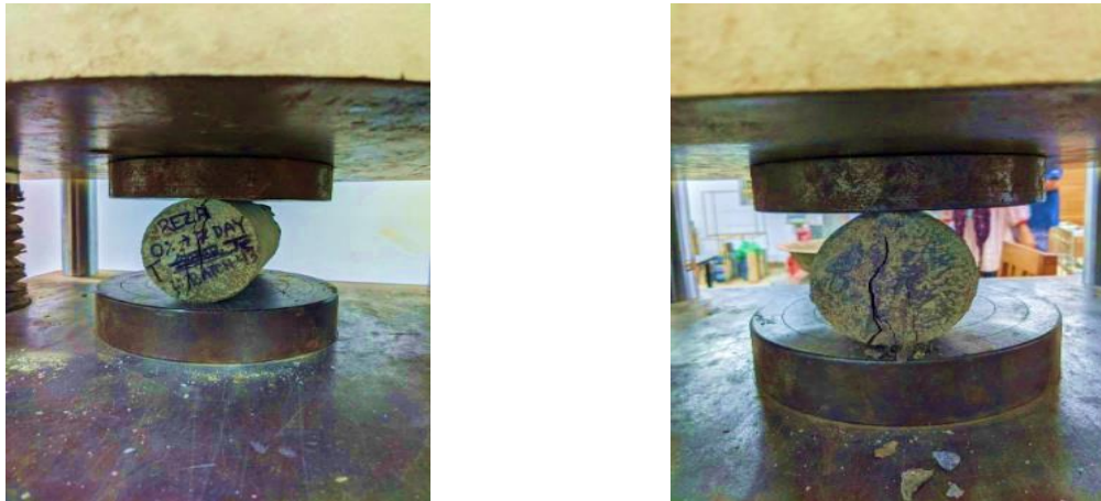
Figure 14. Split tensile strength test
