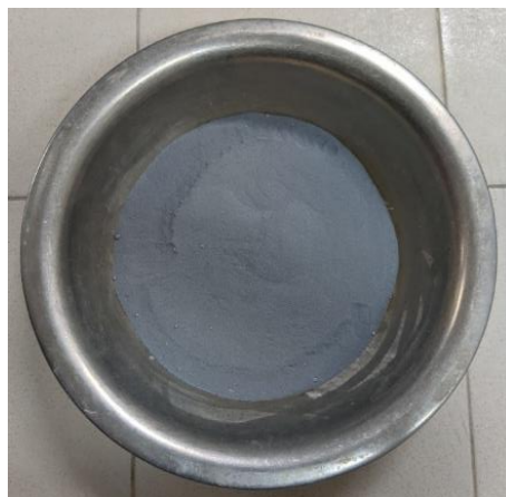
Fig. 7. Micro Silica (Elkem Micro Silica 971)
