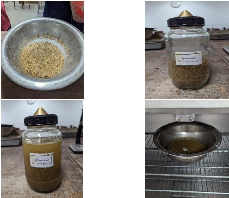
Fig. 6. Specific gravity and absorption capacity of sand
