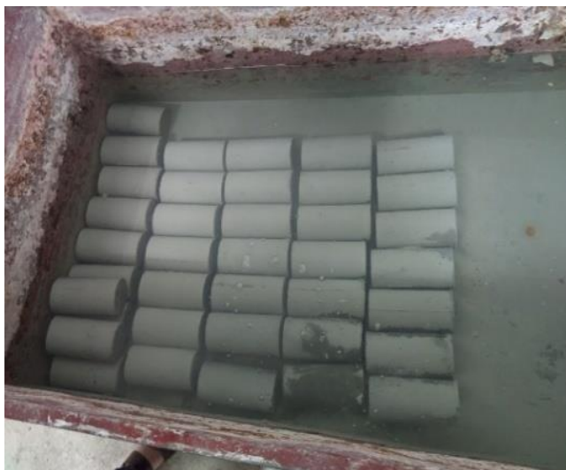
Fig. 11. Curing of some concrete cylinder specimens
