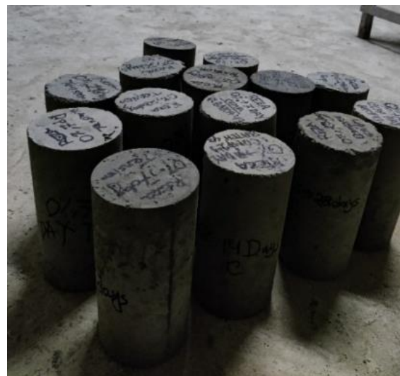
Fig. 12. Concrete cylinder specimen after 28 days of curing
