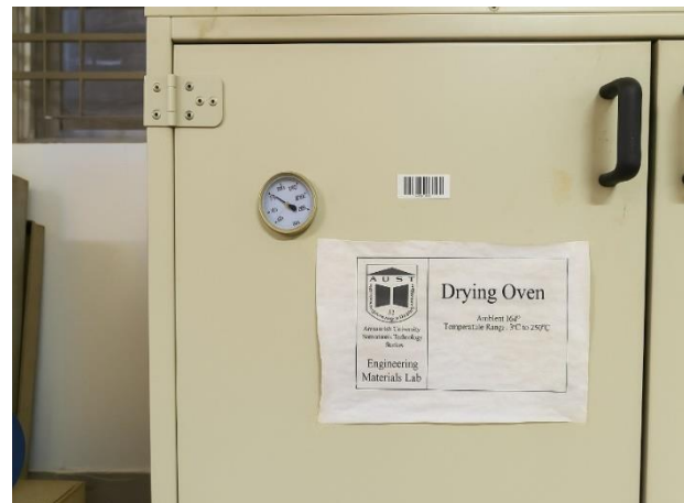
Fig. 15. Oven drying of concrete specimens prior to water absorption testing to ensure consistent moisture removal
