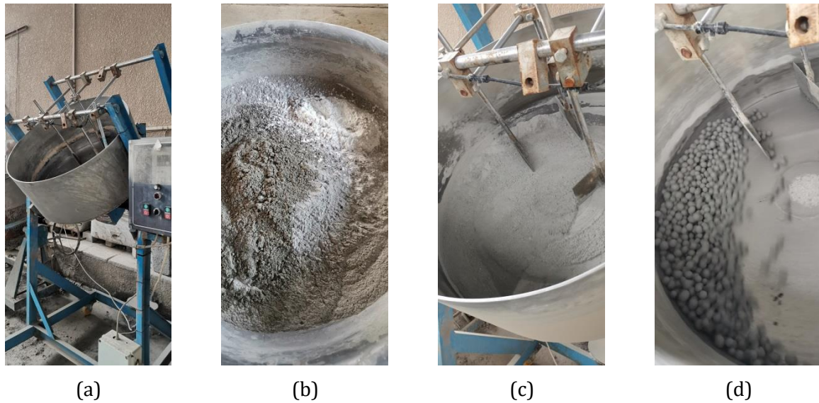
Fig. 4. Steps for manufacturing artificial coarse aggregate via the cold bonding technique (a) Pelletizer disc, (b) Dry powder, (c) Homogeneity of ingredients, (d) Formation of pellets
