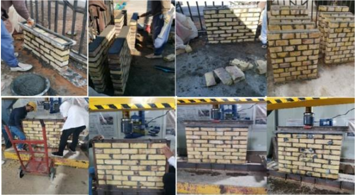
Fig. 4. Construction and setup of walls to test
