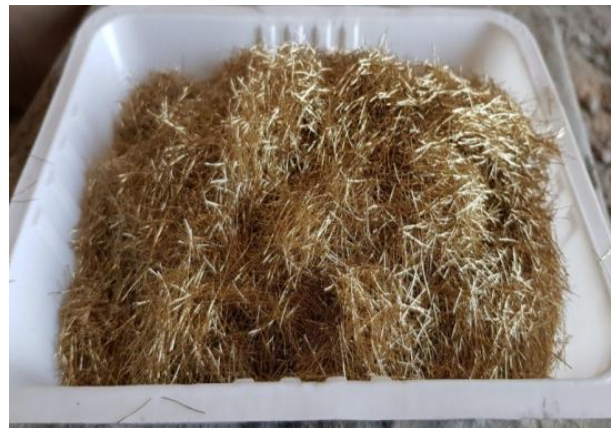
Fig. 3. Steel fibers used in this study
