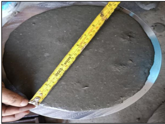
Fig.4. Flow table test of RPC mixtures
