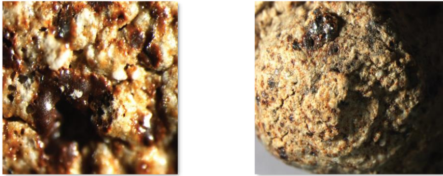
Fig. 4. Microstructure of sintered fly ash lightweight aggregate (10 µm and 1.5x)
