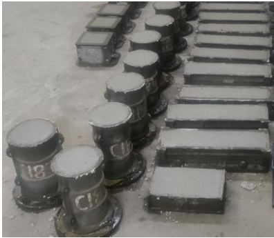
Fig. 5 Concrete cubes, cylinders, and beams in molds
