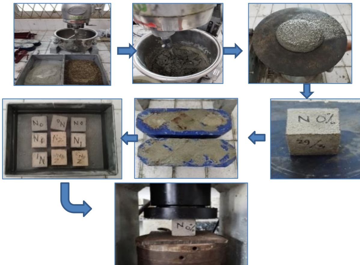
Fig. 2. Test specimen manufacturing procedure
