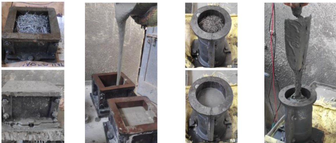
Fig. 6. Manufacturing of SIFCON
