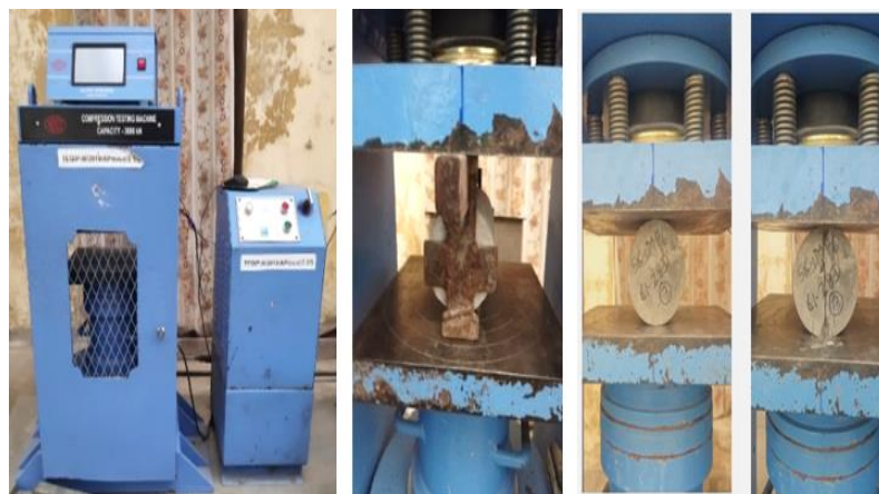
Fig. 8. Test setup of split tensile strength
