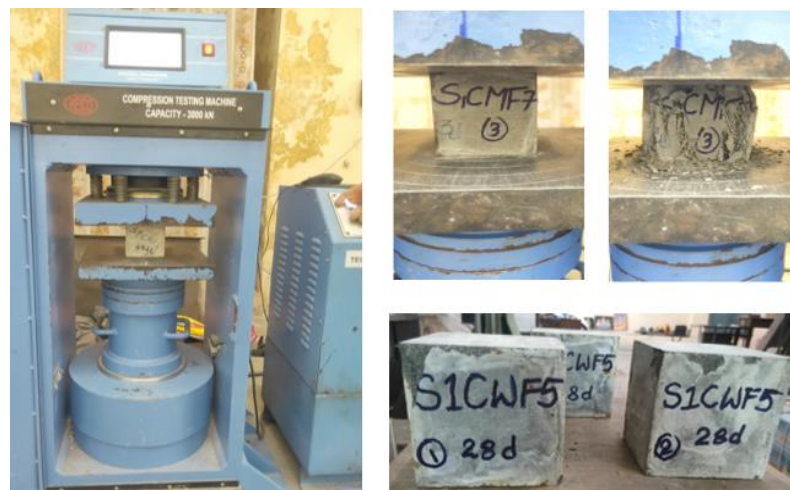
Fig. 7. Arrangement for compressive strength testing
