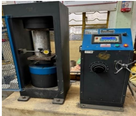
Fig. 3. Setup for stress- strain behavior
