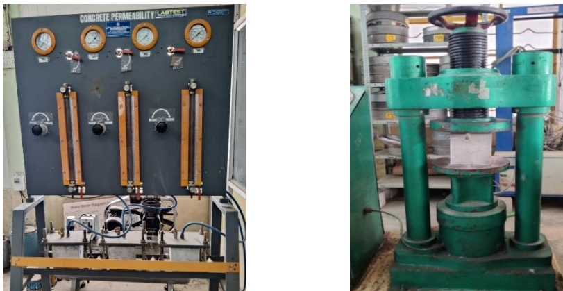
Fig. 5. Concrete permeability test setup
