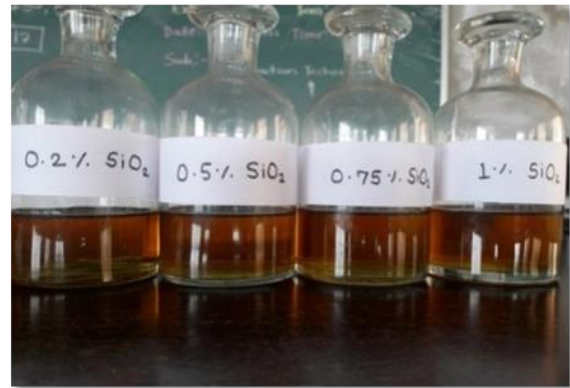
Fig. 4. Simarouba glauca Methyl Ester with \text{SiO}_2 nanoparticles samples prepared for experimentation [19]
