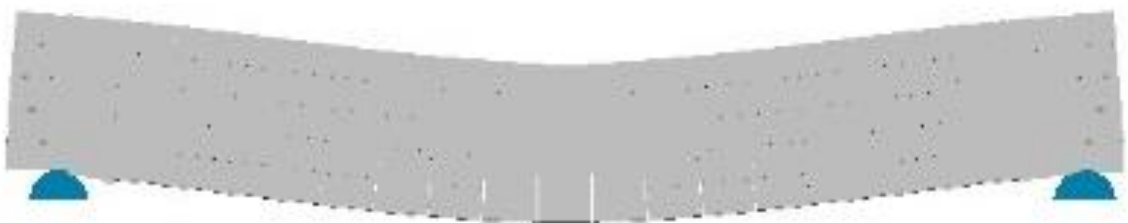
Fig. 16. Crack patterns and deflected shape observed from AEM
