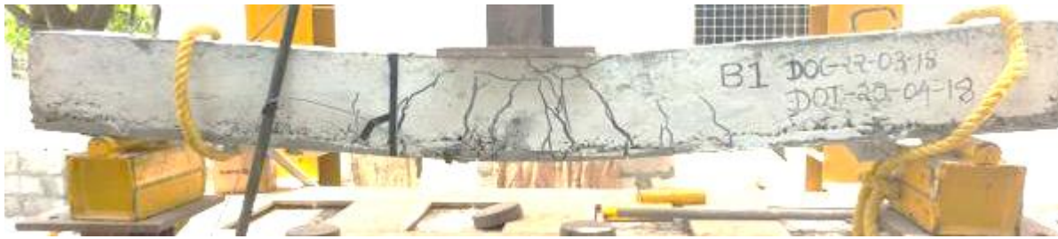
Fig. 13. Crack patterns and deflected shape [12]
