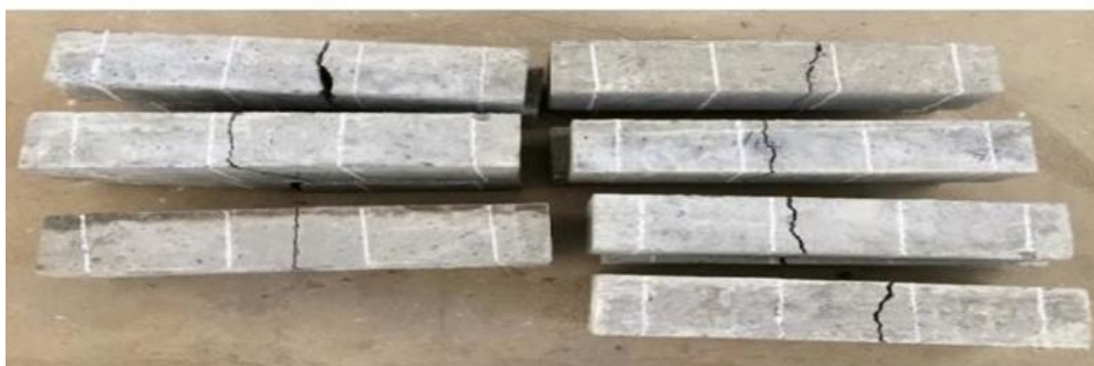
Fig. 9. Typical failures of prisms under flexure
