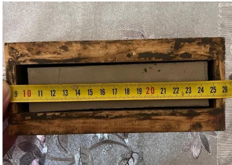
Fig. 6. Illustration of clay shrinkage
