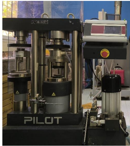
Fig. 3. Controls Pilot Compact-Line for compression strengths
