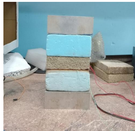
Fig. 5. The hot plane method in the transient regime
