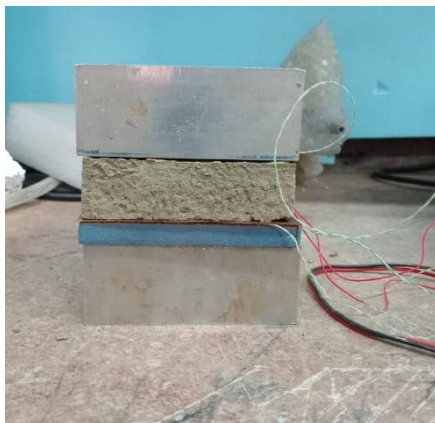
Fig. 4. The asymmetric hot plane method in steady-state device
