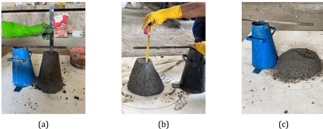
Fig. 10. Slump test: (a) geopolymer concrete base mix (GM12) (b) geopolymer concrete (GM21) mix (c) geopolymer concrete (GM31) mix
