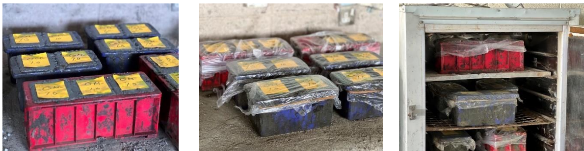
Fig. 7. The steps of curing geopolymer concrete mixes
