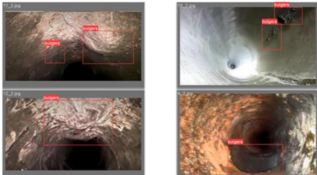
Fig. 7. An example of training a neural network to recognize a bulge-type defects
