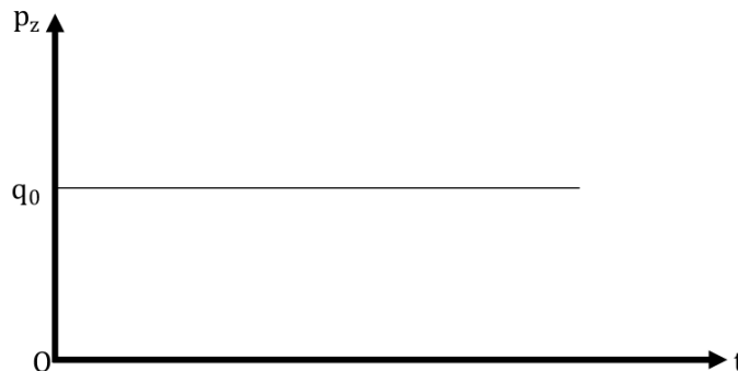
Fig. 3. The sudden transverse dynamic load applied to the FG-BNNT/CF reinforced polymer matrix composite beams
