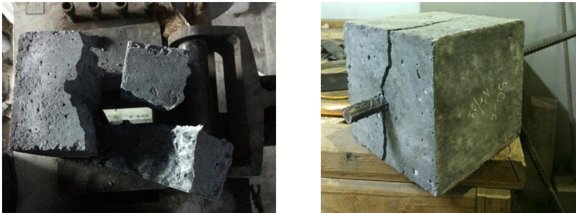
Fig. 5. Failure modes observed after testing
