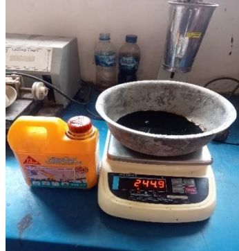
Fig. 5. Superplasticizer admixture used to improve the workability of fiber-reinforced concrete
