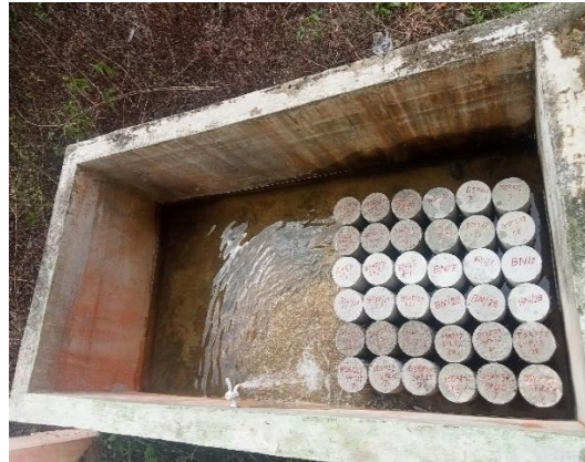
Fig. 7. Curing of concrete specimens in a water tank to maintain hydration and ensure optimal strength development
