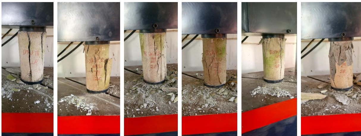
Fig. 8. Compressive strength testing of concrete cylinders using a Universal Testing Machine (UTM) as per [62] standards
