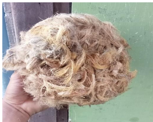
Fig. 4. Areca catechu fiber after processing, cut into lengths of 30–50 mm before being used in the concrete mixture
