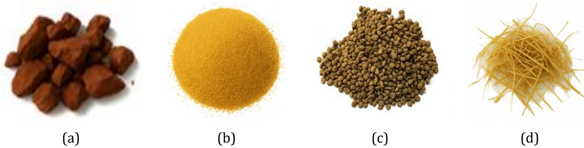
Fig. 3. Raw materials for manufacturing raw clay bricks (a) Clay (<math><0,075\text{mm}</math>), (b) Dune sand (<math>0-2\text{mm}</math>), (c) Coarse sand (<math>2-2.5\text{ mm}</math>), and (d) Straw fiber (<math>25-30\text{ mm}</math>)
