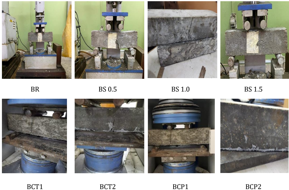
Fig. 7. Failure mode of tested specimens
