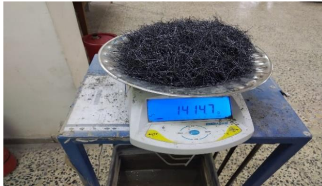
Fig. 1. Steel fiber used in specimens
