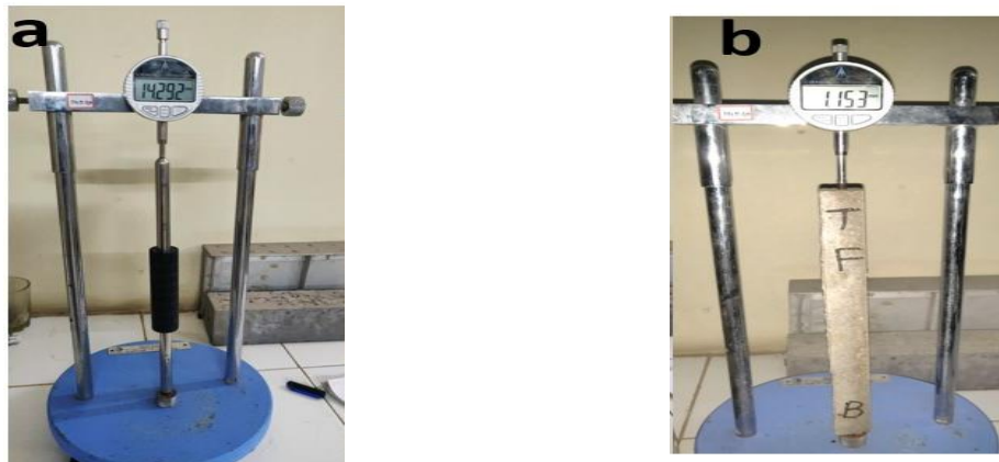
Fig. 5. (a) Reference rod and (b) testing specimen
