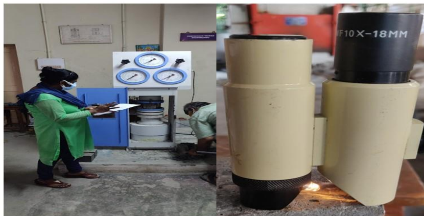
Fig. 6. Cracks inducing on the specimens using a CTM and b. Microscope used for the crack closure assessment
