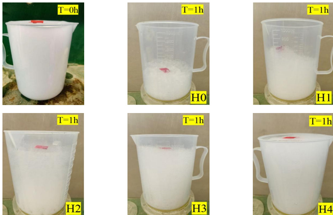
Fig. 2. The stability of foam with different HEC content in air
