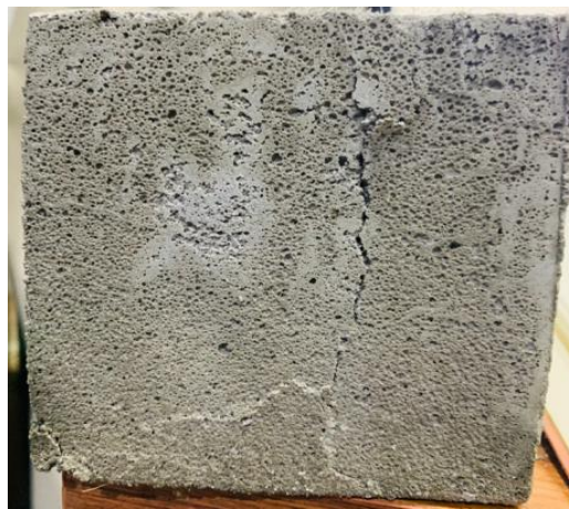
Fig. 7. Failure pattern of specimen
