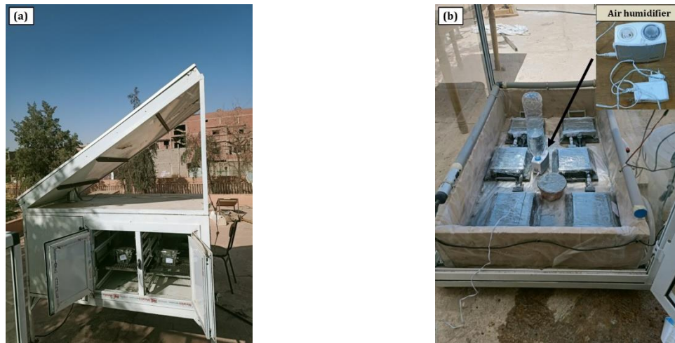
Fig. 3. Heat treatment system (solar radiation drying): (a) SD, (b) SG
