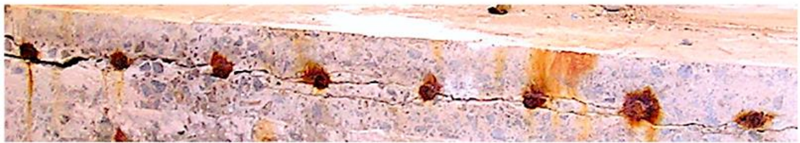
Fig. 1. Cut cross-section in 2009 of a 450 mm thick deck slab (cover 40 mm) exposed since the 1930s in the Newcastle Harbour marine atmosphere, showing delamination crack passing through the bottom of the 16 mm diameter bars. R.E. Melchers 2009 [2]
