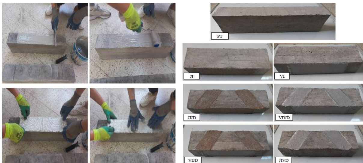
Fig. 5. Application of FRP strengthening systems and layout of tested configurations: bottom-only, U-wrap, and hybrid reinforcement schemes
