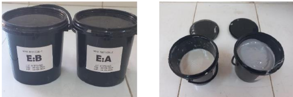
Fig. 1. Two-component NOVA MASTICOLLE epoxy adhesive system used for bonding FRP sheets: Component A (resin) and Component B (hardener)
