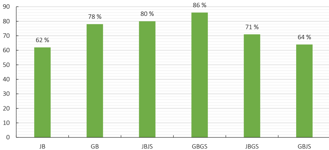
Fig. 12. Percentage gain in ductility index for all strengthened beams compared to the unstrengthened referenc.
