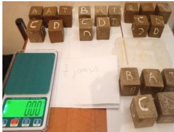
Fig. 14. Measurement of mass loss
