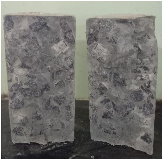
Fig. 12. Damaged NMA 100% RA cylinder
