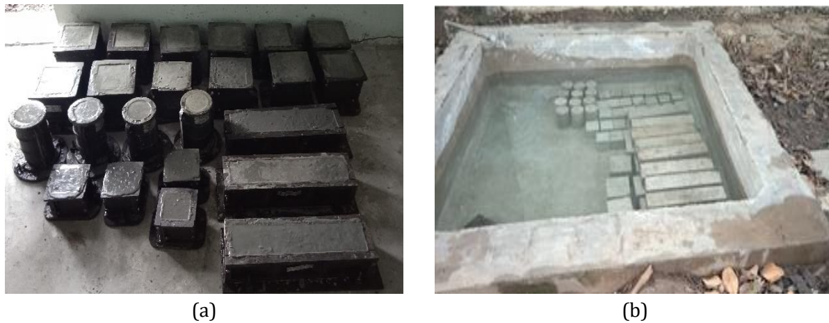
Fig. 1. (a)Casted samples and ( b) Curing of samples in the curing tank
