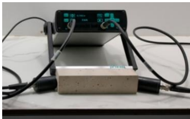
Fig. 7. Non-destructive measurement of dynamic modulus of elasticity ( E_d ) via ultrasonic pulse velocity
