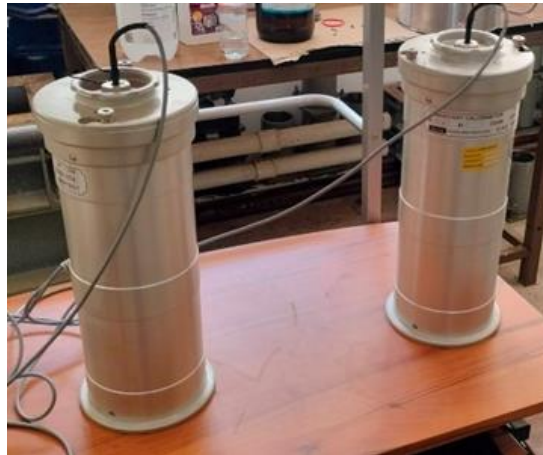
Fig. 5. Semi-adiabatic hydration heat monitoring using a Langavant calorimeter
