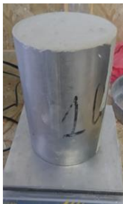
Fig. 4. Fresh density measurement using a calibrated cylindrical container
