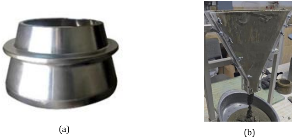
Fig. 3. Rheological property measurement: (a) Mini-slump cone; (b) Mini V-funnel apparatus
