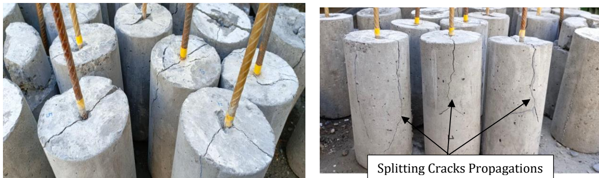
Fig. 6. failure modes of the examined specimens
