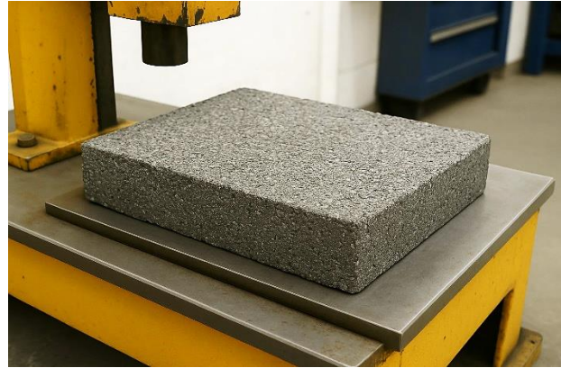
Fig. 11. Hamburg wheel-track sample
