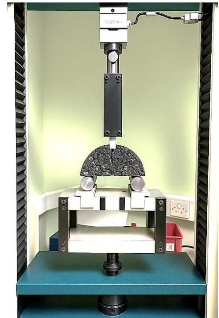
Fig. 30. Crack length recording under three-point bending test
