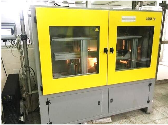
Fig. 10. The apparatus of Hamburg wheel-track
