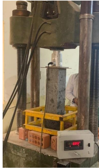
Fig. 7. RC column specimen inside the universal testing machine
