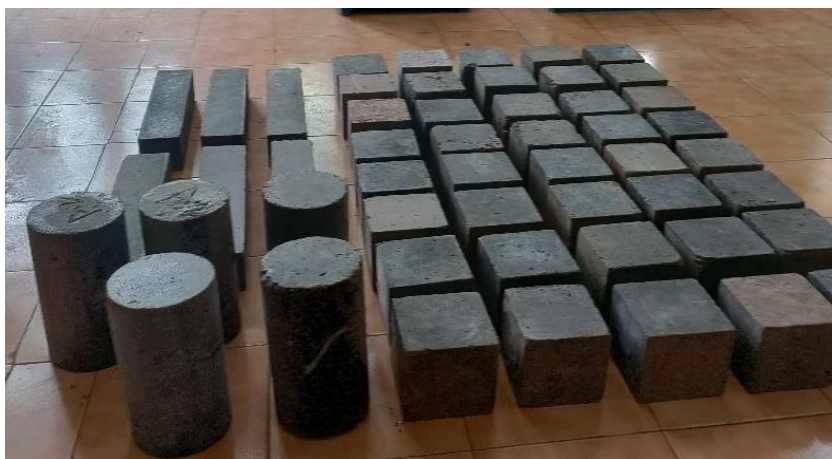
Fig. 2. Concrete samples prepared for strength testing
