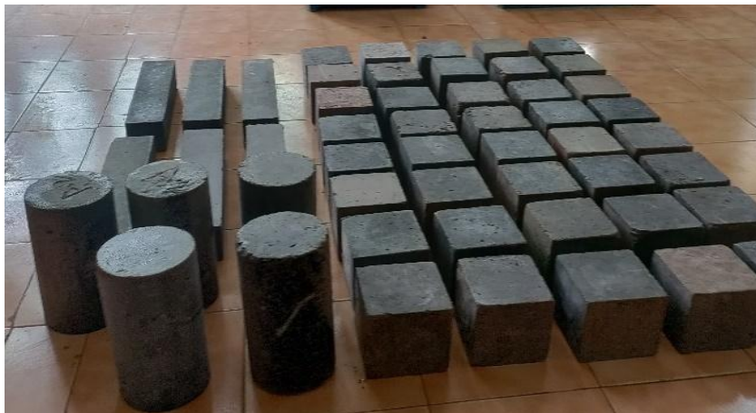
Fig. 2. Concrete samples prepared for strength testing
