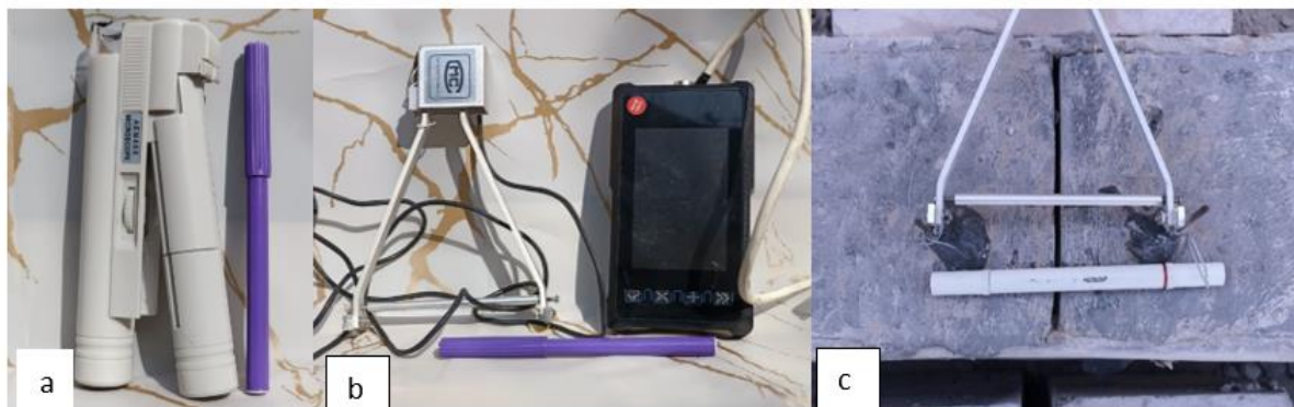
Fig. 5. (a) Crackmeter, (b) and (c) the extensometer installation
