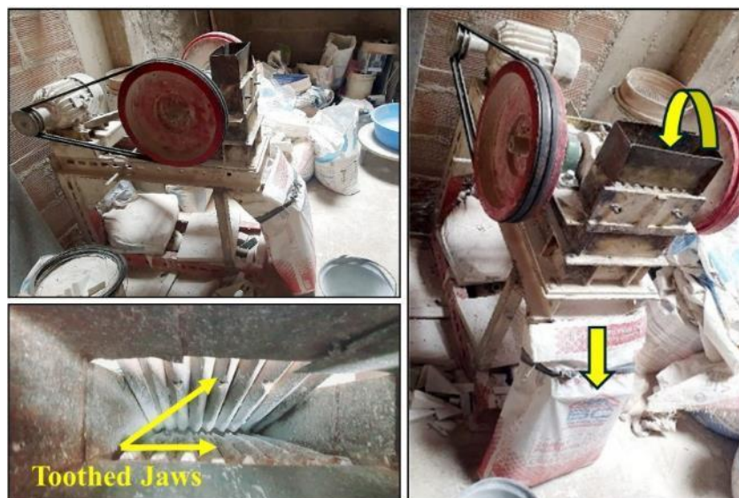
Fig. 1. Toothed jaw crusher used for crushing aggregates
