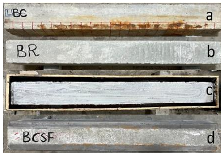
Fig. 2. (a) Side view of corroded beam (b) Top view of reference beam (c) Epoxy coating beam before casting (d) Top view of strengthened beam with FRSCC
