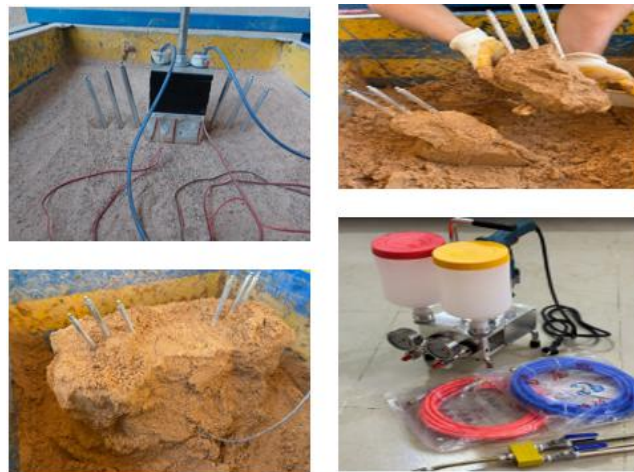
Fig. 7. The pipes injection and the PU machine.
