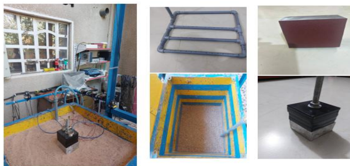
Fig. 4. The footing, water distribution system, frame, and steel box
