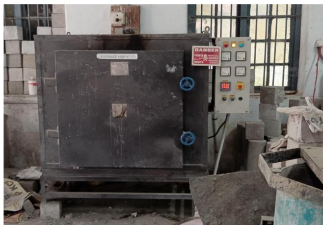
Fig. 1. Bogie Hearth furnace setup for heating specimens up to 500°C
