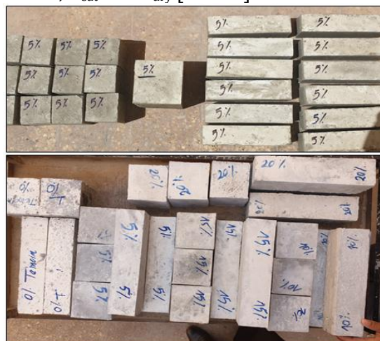
Fig. 4. Photographs of the cubic and prismatic samples
