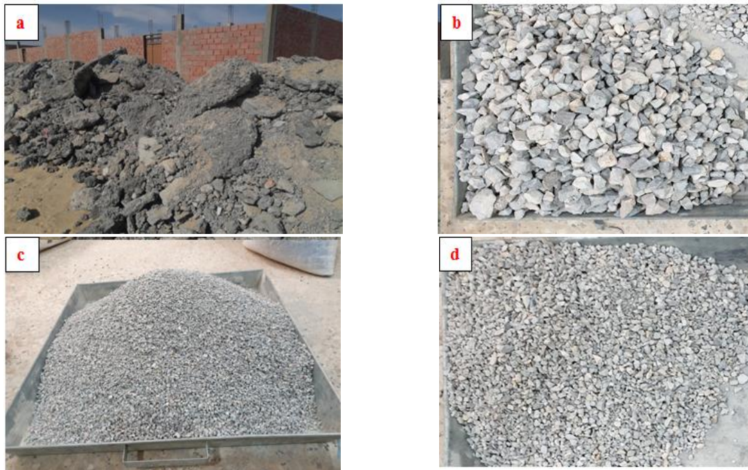
Fig. 2. a) Demolished concrete, b) RG 10/16, c) RS 0/5 and d) RG 5/10
