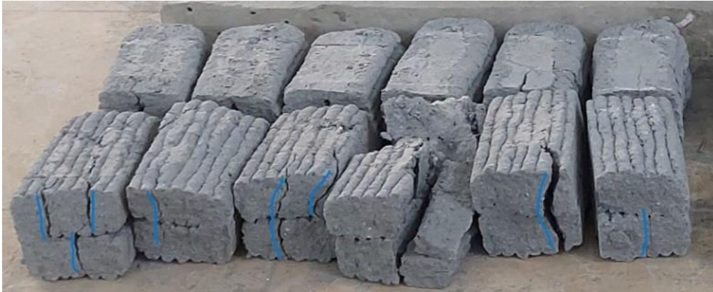
Fig. 19. Cracking pattern in Y loading orientation
