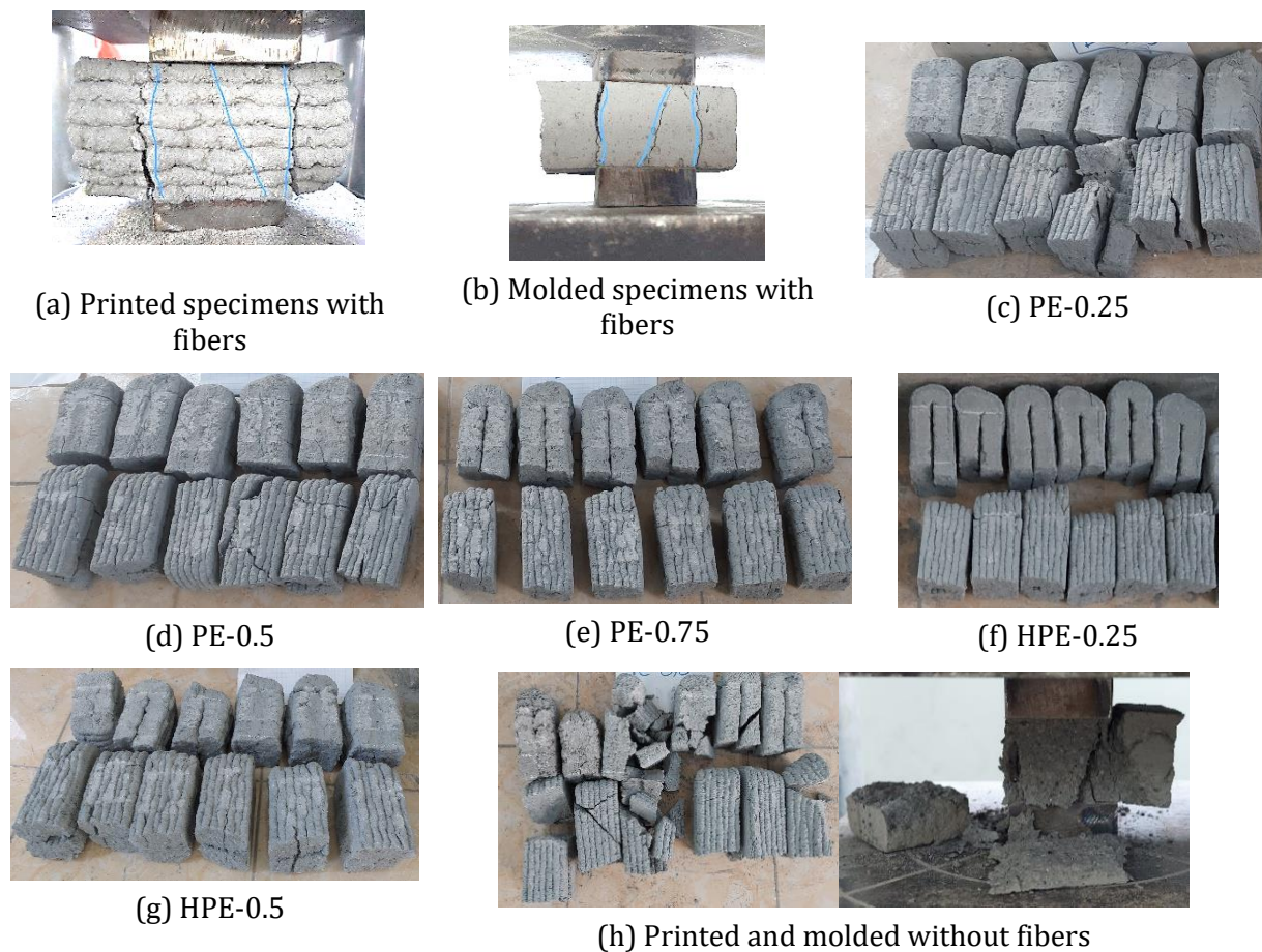
Fig. 11. Compression cracking patterns
