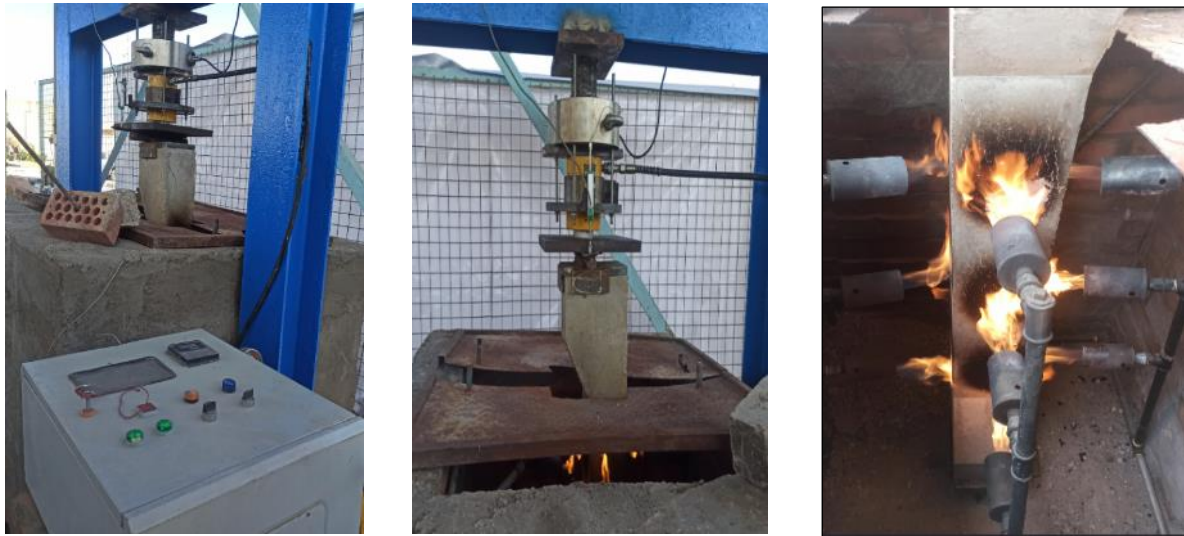
Fig. 5. Specimens subjected to fire exposure under pre-loading curve
