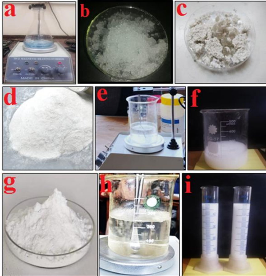
Fig. 5. (a) preparation of silica gel, (b)(c) silica gel, (d) \text{SiO}_2 nanoparticles powder, (e)(f) Nanocomposite of \text{SiO}_2 nanoparticles and paraloid B-72, (g) \text{Ca}(\text{OH})_2 Nanoparticles, (h)(i) Nanocomposite of \text{Ca}(\text{OH})_2 nanoparticles and paraloid B-72
