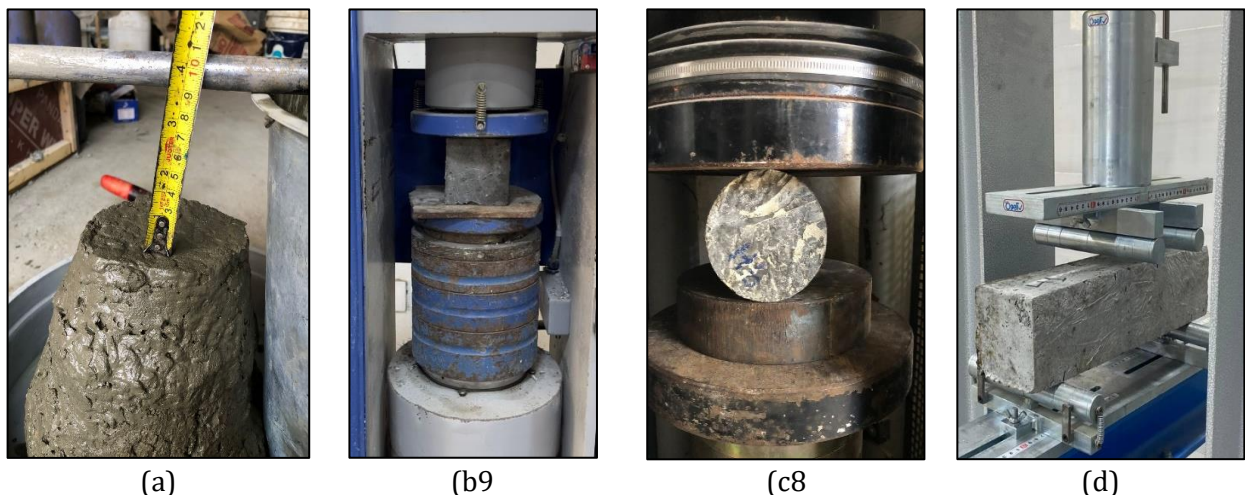
Fig. 3. (a) Workability test (slump test), (b) concrete strength test (compressive), (d) flexural strength test (two-point loading), (c) tensile strength test (splitting method)
