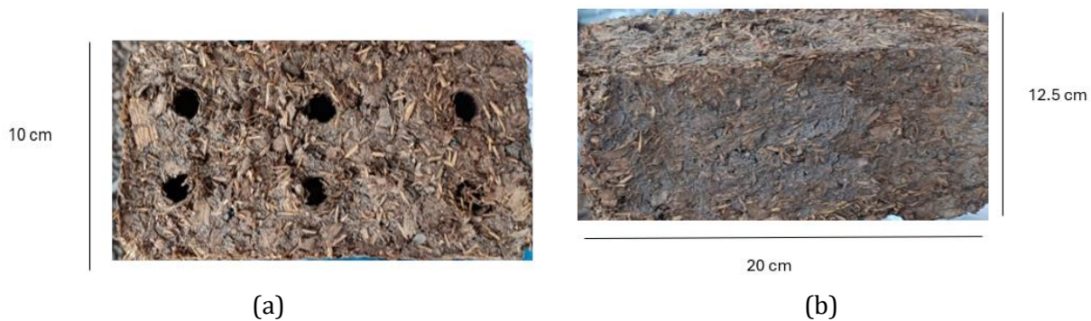
Fig. 1. Geometry and appearance of the produced briquette: (a) top view (left) showing surface perforation holes; (b) side view (right). Nominal dimensions are 20 cm × 10 cm × 12.5 cm (length × width × height)
