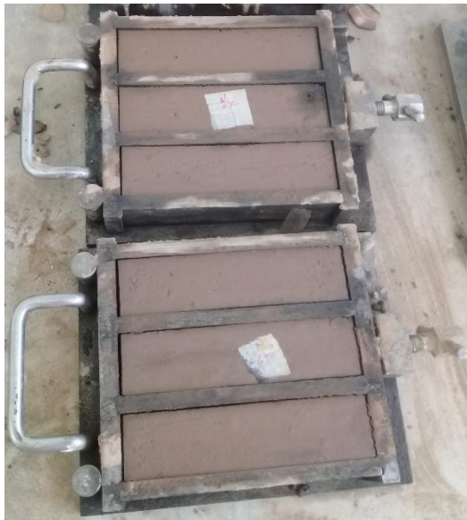
Fig. 3. Photograph of fresh molded earth block
