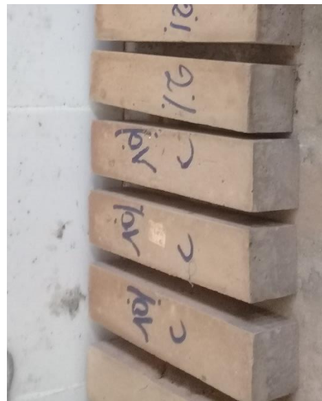
Fig. 4. Photograph of hardened earth block
