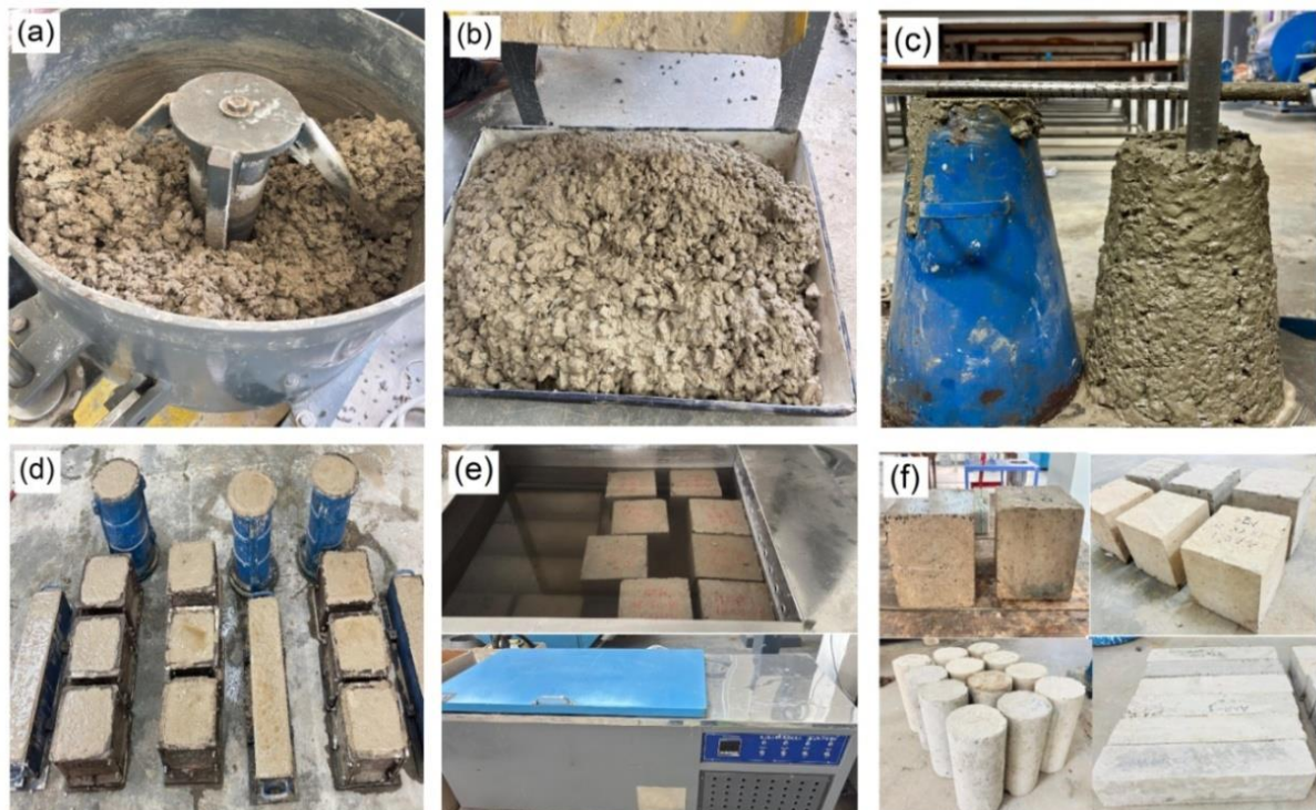
Fig. 2. Freshly prepared concrete mixture, the slump cone test, and prepared test specimens
